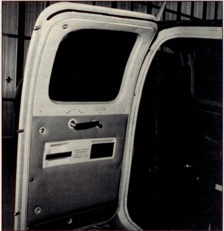
Massive locking pins on aft door help ensure pressure vessel integrity. When loading passengers or cargo, pilot must make sure the rear door seal is not damaged and the door is locked properly.
