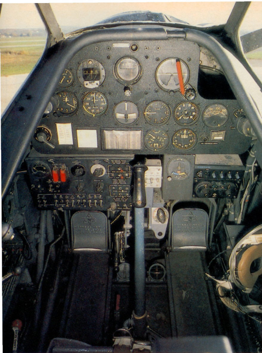
The Harvard's roomy cockpit matched wartime military "standardization" criteria, but even within the type, no two panels were necessarily the same. Bryce's MKIII has provision for a .30 cal machine gun, but not for a standard "civilian" panel.
