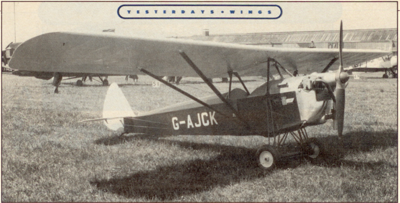
The improved 1930 Super Parasol also was known as the V-Parasol because of its V-struts. Plans for this improved version were serialized in Popular Aviation magazine in 1930. The aircraft shown above was built in England and has modified landing gear and a British-built 36-hp Aeronca E-113 engine. continued and significantly for use in an aircraft.
