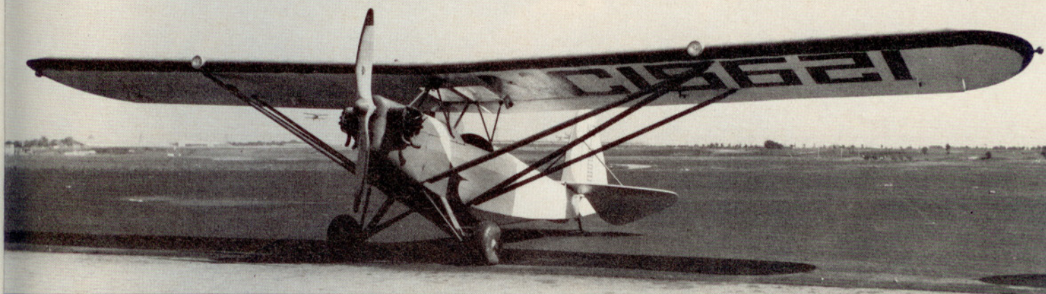
A major design change was necessary in order to qualify the basic Heath Parasol for an Approved Type Certificate. The most obvious new features, shown above left, on the LNB-4 are the increased wingspan, larger tail and revised strut arrangement. The LNB-4 had the Heath B-4 engine. The LNA-40 above right was built from plans available through the Experimental Aircraft Association, 66 years after the first one flew. The Heath LNA-40, bottom, had noticeably different nose contours; because of the clockwise A-40 engine, the hinge-down door was relocated to the right on this aircraft.
