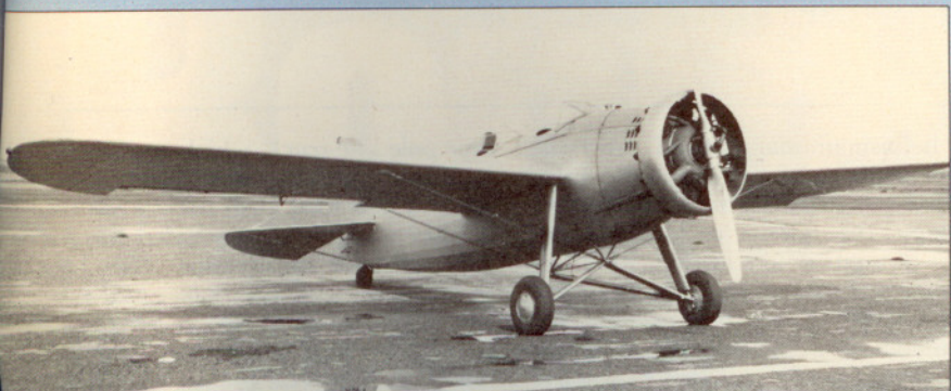
The original B-7 and B-7C did not sell. The single Emsco B-7C, above, had improved cockpits and windshields and a "speed ring" around the radial engine.
