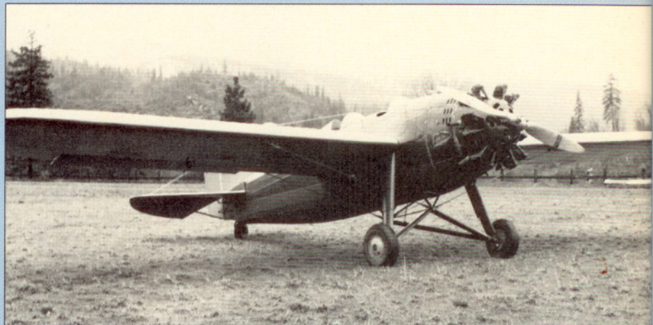
The final version of the Emsco Mid-wing was the B-7CH. A Curtiss Challenger engine replaced the Continental and Wright J-6-5 Whirlwind of earlier models.
