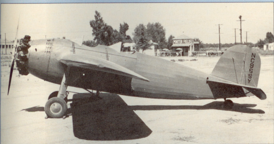
The single B-7C at Van Nuys, Calif., in later years. Note the large number of stringers used to round out the square fuselage frame and deletion of cowling.
