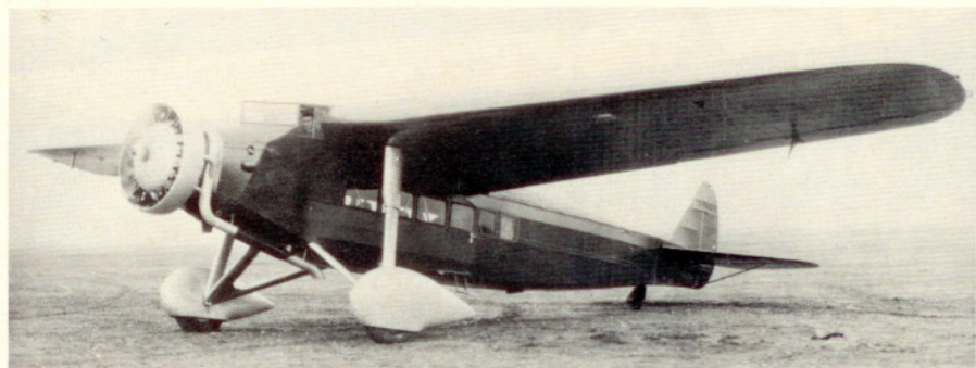
Just a little rearrangement made the single Fokker F-14A look like an entirely different design. The wing has been lowered to the top of the fuselage and the pilot has been moved into a closed cabin up front. The addition of antidrag rings to radial engines became a common practice from 1930 on.
