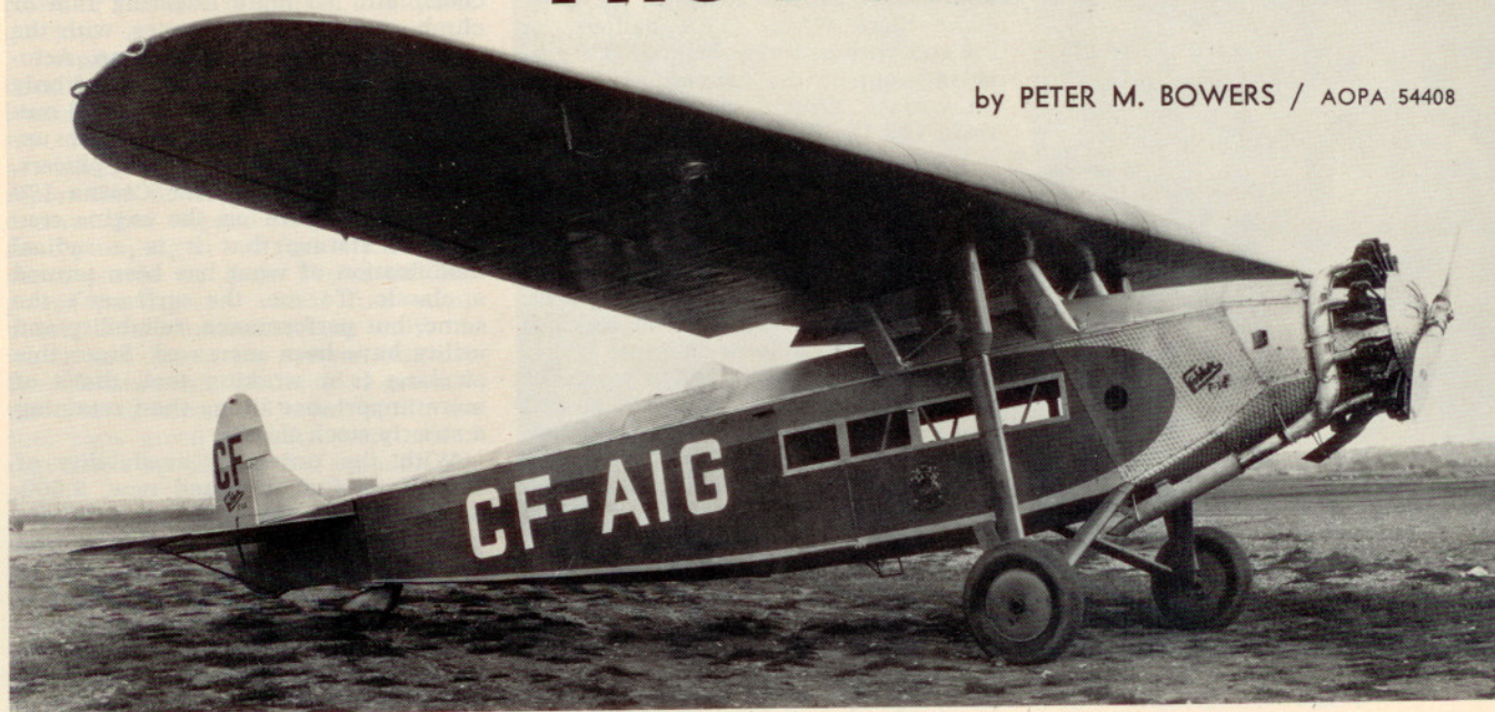
The Fokker F-14 was developed for Western Air Express and the prototype shown here carried Western markings before being sold to Canada. The parasol wing position was used to minimize visibility problems resulting from the location of the pilot's open cockpit.
