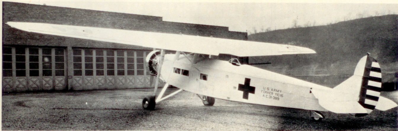
The ninth airplane of the 20-plane Army Y1C-14 contract was converted to the Y1C-15 aerial ambulance at the factory and was delivered in this special white color scheme. The Army then bought the last civil F-14 and had it converted to an ambulance similar to the C-15A.
