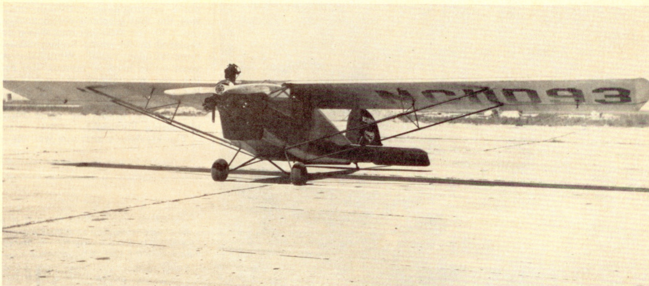
The squat Alexander Flyabout was designed expressly to meet the general aviation marketing conditions following the Great Depression. Good performance on low horsepower was achieved with long, gliderlike wings. This is the D-2 model, powered by the 45-hp Szekely radial engine. Author's photos.
